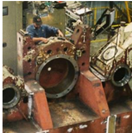
Specialised machining and line boring
