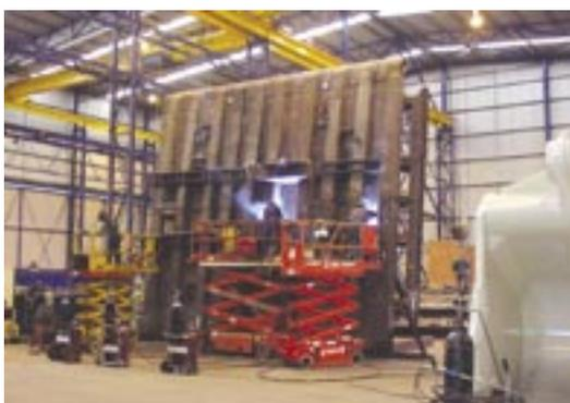
Fabrication of dump truck body at John's Engineering
