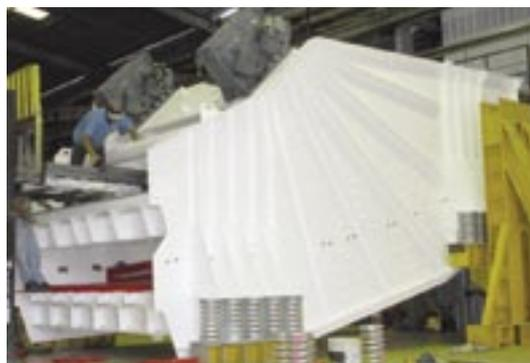
Vibrating screen manufactured for Ludowici Mineral Processing Equipment Pty Ltd
