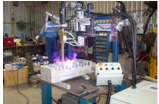
Testing of Narrow Gap Welding processes
