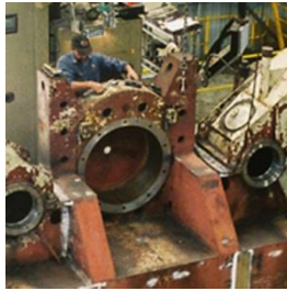
Specialised machining and line boring
